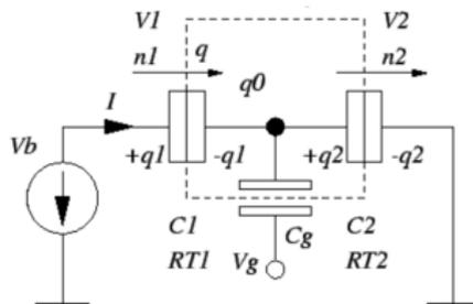
Figure: SET transistor.<sup>13</sup>
