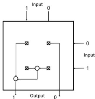
Figure: Brownian NAND constructed from a  $2 \times 2$ -CJoin and two Hubs.
