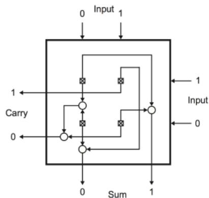
Figure: Brownian half-adder constructed from a  $2 \times 2$ -CJoin and four Hubs.<sup>11</sup>
