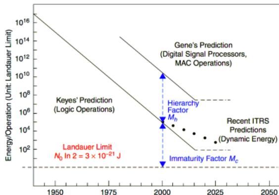
Energy per operation w.r.t. the Landauer limit at room temperature for transistor-based devices.<sup>2</sup>
